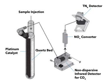
Figure 2. Schematic of TN<sub>b</sub> Analysis Performed with the 1080 TOC Analyzer
